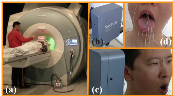
Figure 3: Experiment setting for data acquisition. (a) the SIEMENS MRI system. (b) NDI Wave EMA system. (c) Gathering the articulatory movement data using EMA. (d) Placing EMA coils on the tongue.
