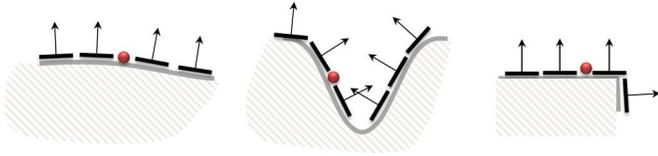
Fig. 5. Left: the normal directions of triangles close to a vertex (shown as a red sphere) on a smooth pavement surface are mostly in parallel. Middle: when it is close to a crack, normals are irregularly scattered. Right: a non-uniform normal distribution does not necessary mean sharp vertex.
