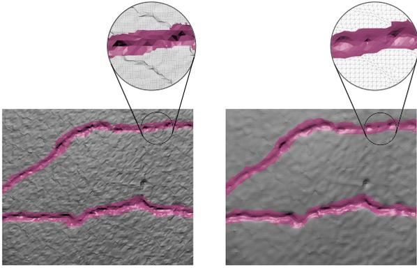
Fig. 11. Side-by-side results of the crack detection with the proposed algorithm using LIDAR (left) and Kinect (right) data.
