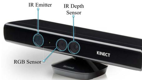
Fig. 1. The first generation of Microsoft Kinect sensor.
