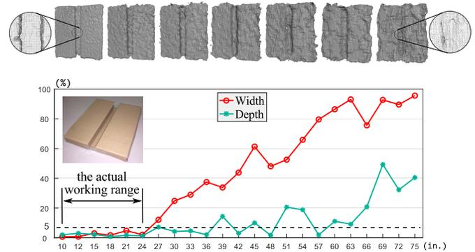
Fig. 10. In the phantom study, we test the accuracy of the proposed algorithm using a standard man-made cracking surface. While the relative error goes up when the Kinect moves further and further away from the phantom surface, the accuracy of our algorithm is typically below 5% if the Kinect-phantom distance is between 10 to 30 inches, within which is how our data collection was set. The reconstructed surfaces are also given in top.
