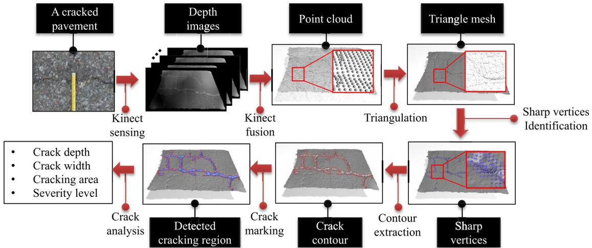
Fig. 3. An overview of the proposal framework of crack analysis.
