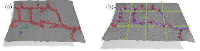
Fig. 7. (a) The result of BFS on a pavement mesh. The red regions are the large connected component. Other small components in other colors are discarded. (b) Crack depth evaluation by grids. At each grid, the deepest sharp vertices are picked (red spheres) for local depth evaluation.
