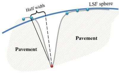
Fig. 8. Width measurements.
