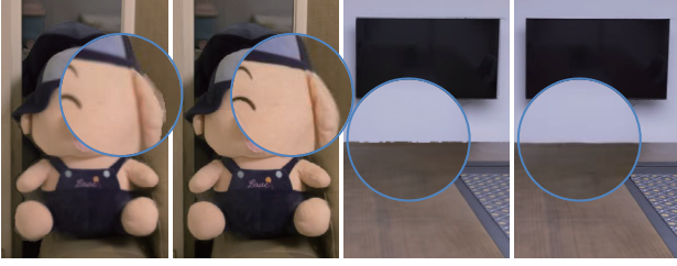
Fig. 13. View warping vs. DSRNet. For each pair, the image on the left is produced by our view warping algorithm, and the image on the right is produced by the DSRNet. The blurring and aliasing at object boundaries are effectively removed by the DSRNet.
