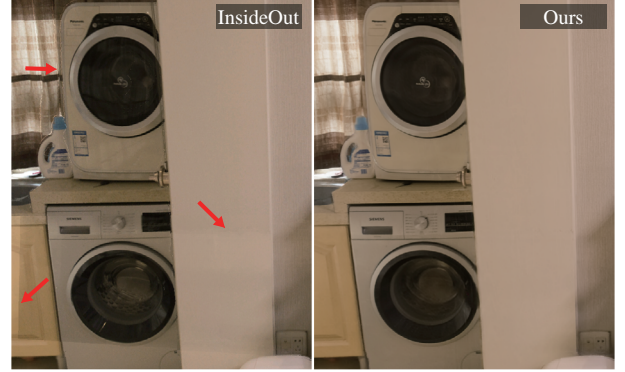
Fig. 5. Compared with InsideOut[Hedman et al. 2016], our view warping can avoid discontinuity artifacts and produce smoother image blending result.
