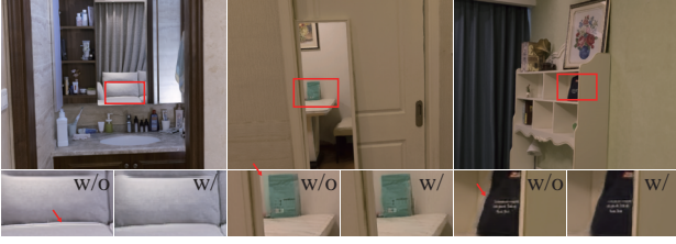
Fig. 14. The improvement of object boundary rendering quality using the MVR module. W/: with MVR. W/O: without MVR.
