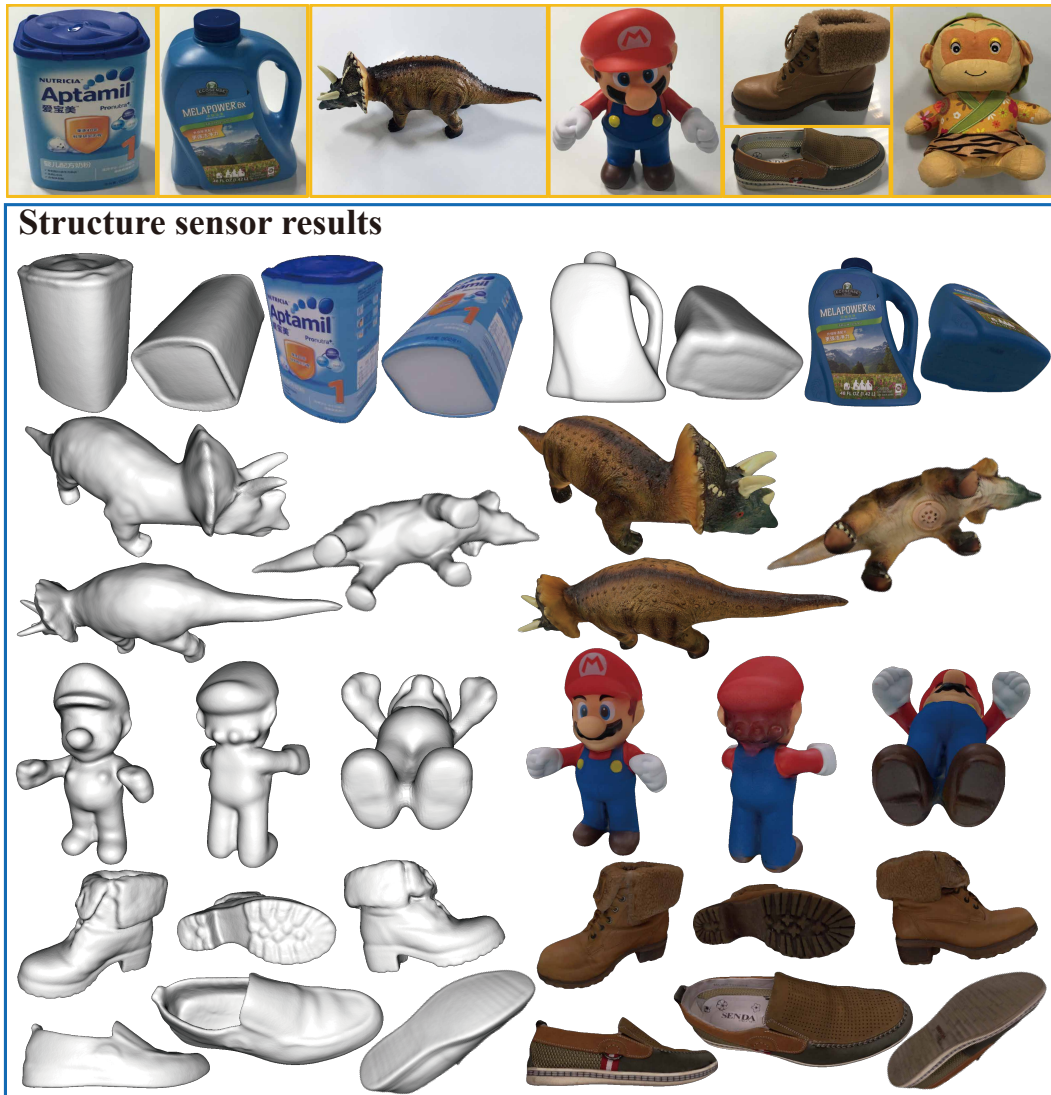
Figure 14: Our system can produce high-quality 3D reconstruction for various objects using Occipital structure sensor. It is robust for geometric-complex items like the toy dinosaur and various shoes. The photometric metric further improves the texture quality. Even the ingredient information on the formula canister is legible.
