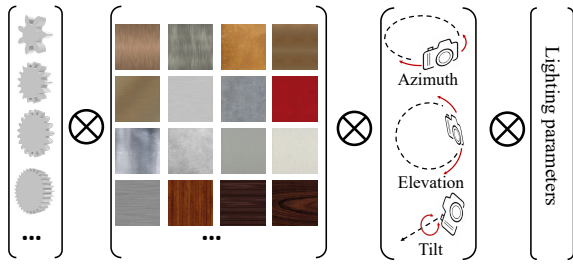
Figure 7: In order to have sufficient training data for the ResNet, we generate over 1.1 millions synthetic 2D images by rendering 3D part models of different parameters with various textures, lighting and camera poses.
