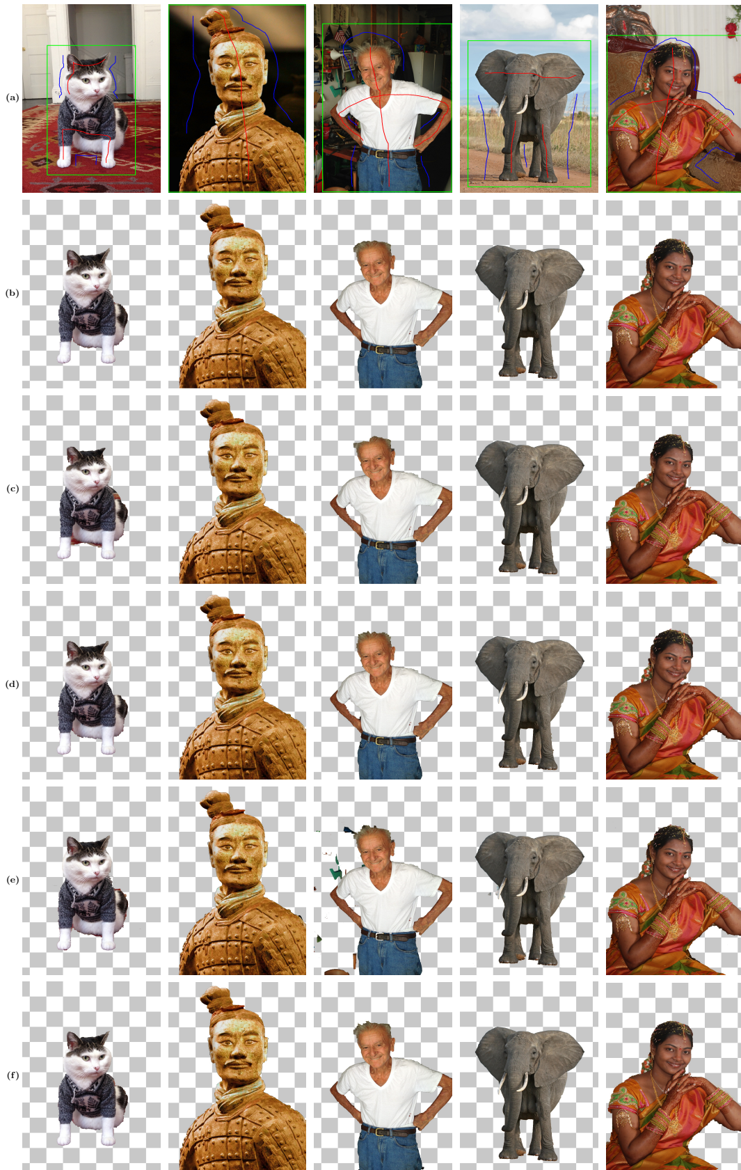
Figure 9: A comparison of results from the different image segmentation algorithms: (a) Original image with user input strokes. (b) Ground truth. (c) Graph Cut. (d) Lazy Snapping. (e) Grabcut. (f) Our method.
